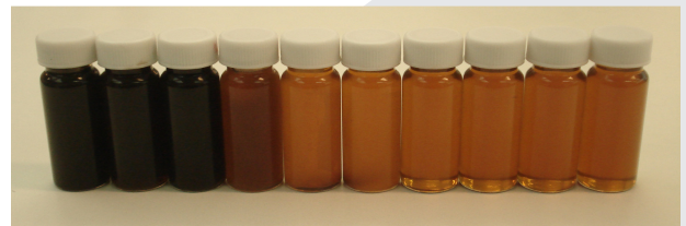
Oil samples with different ages, ranging from a brand new Veritas 800 Marine (right) to a old Veritas 800 Marine oil (left)
